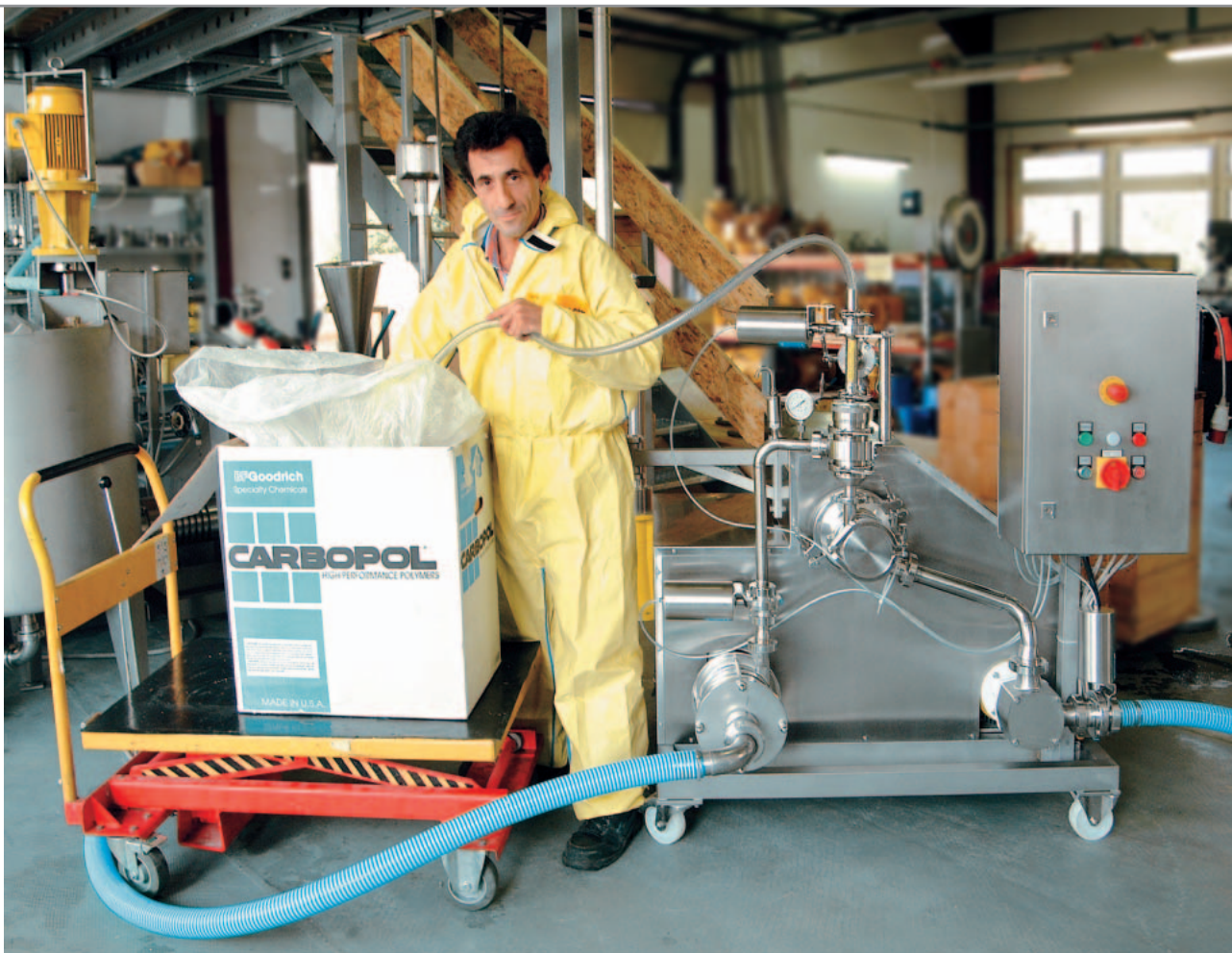
YTRON-PID in a mobile construction Application: Dust-free incorporation of an Acrylic Polymer from a bag to produce a Cosmetic Product
