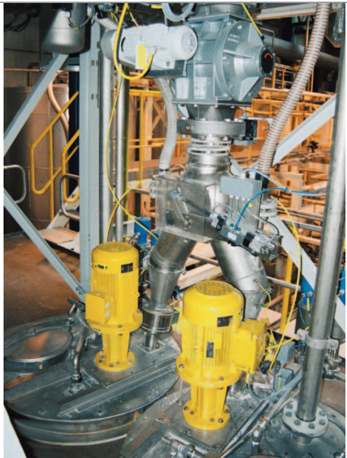
YTRON-Y ByPass in the Brewing Industry Application: Suspending of Diatomaceous Earth CO 2 inerting for a Continuous Discharge of the Product.
