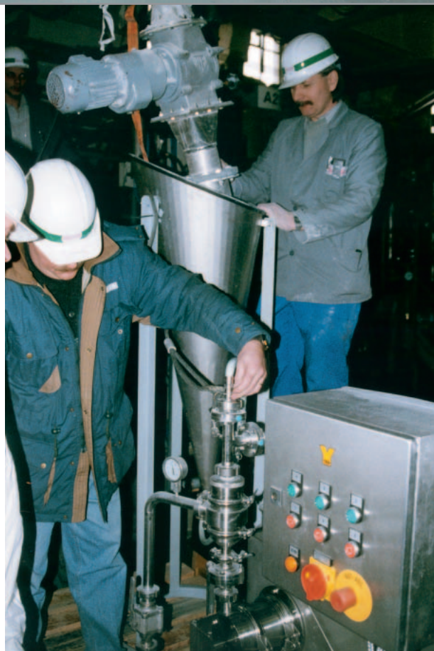
YTRON-PID Powder addition via hopper or from BigBag or silo Application: InLine-dissolution of Poly-Vinyl Alcohol (PVA)
