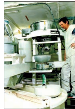
Compact Sieves are suitable for screening wet materials as shown here at Royal Crown Derby.
