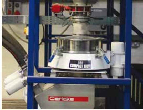
Figure 1. One of the Russell Compact Sieves® installed below a hopper at Altro. • Easily stripped down and cleaned without tools. • Solid rubber suspension provides quieter operation. • High throughput rates offering 10,000 tonnes a day.
